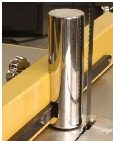
The table tilts using this large handwheel (left) that operates a gear drive. The massive solid steel resaw post (right) is included!
