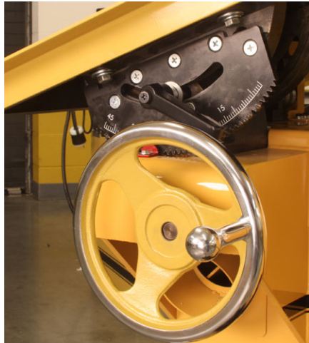
The table tilts using this large handwheel (left) that operates a gear drive. The massive solid steel resaw post (right) is included!
